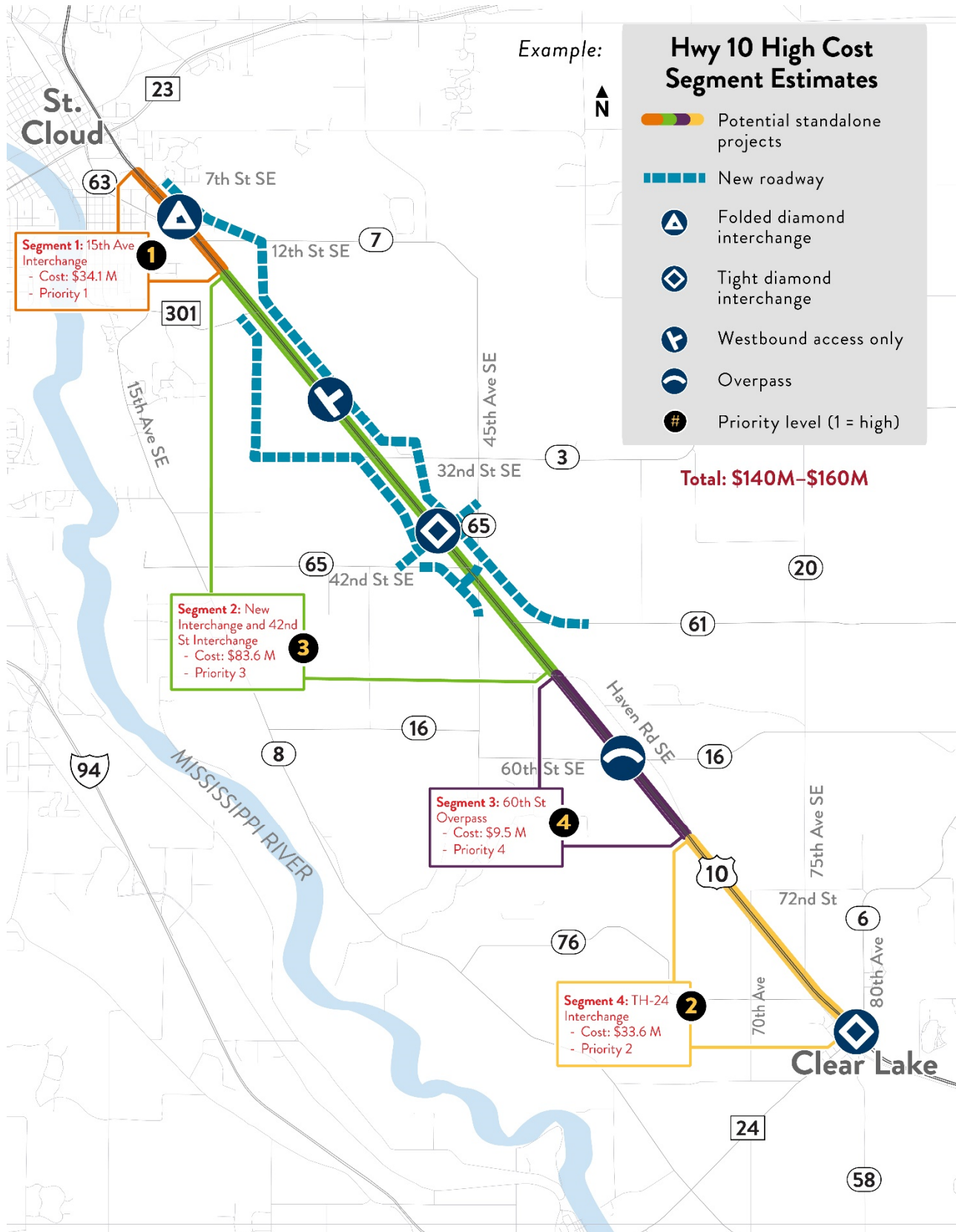
Figure 5: Recommended Higher-Cost Alternative C Independent Buildable Segments
