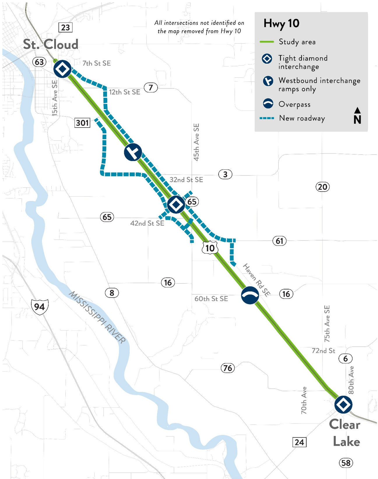
Figure 8: High-Cost Alternative A – Existing Interchange Locations
