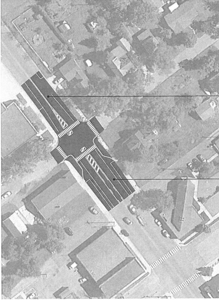
Proposed Cross Section for Main St at 2nd Ave SE, NE leg 42' Curb to Curb
