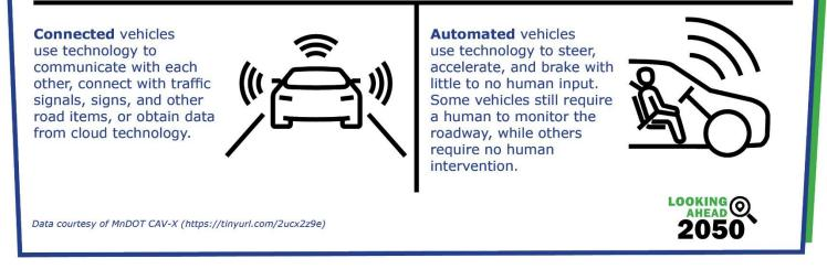
Figure 4.9: Differences between connected and automated vehicles.
