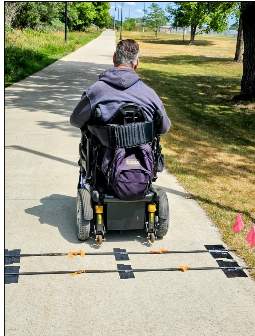
Figure 3.8. A person in a motorized scooter rolling over an active transportation counting tube.
