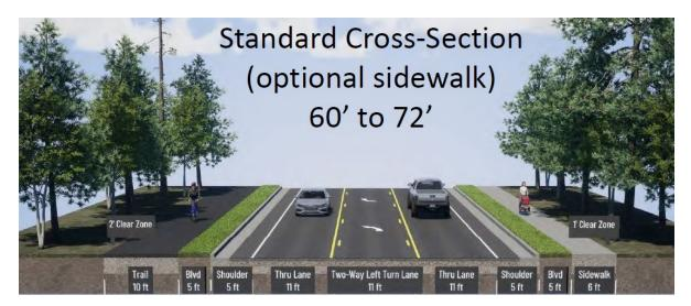
The public was somewhat split on the desire for a sidewalk on the opposite side from the multi-use path. The County has about 66' of right-of-way through the corridor. The roadway and multi-use path require about 60' of space. Sidewalk could be added where space permits and where impacts to property could be minimized.
