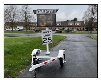
*Figure 52. Example of a portable speed trailer. \*Photo courtesy of All Traffic Solutions.*
