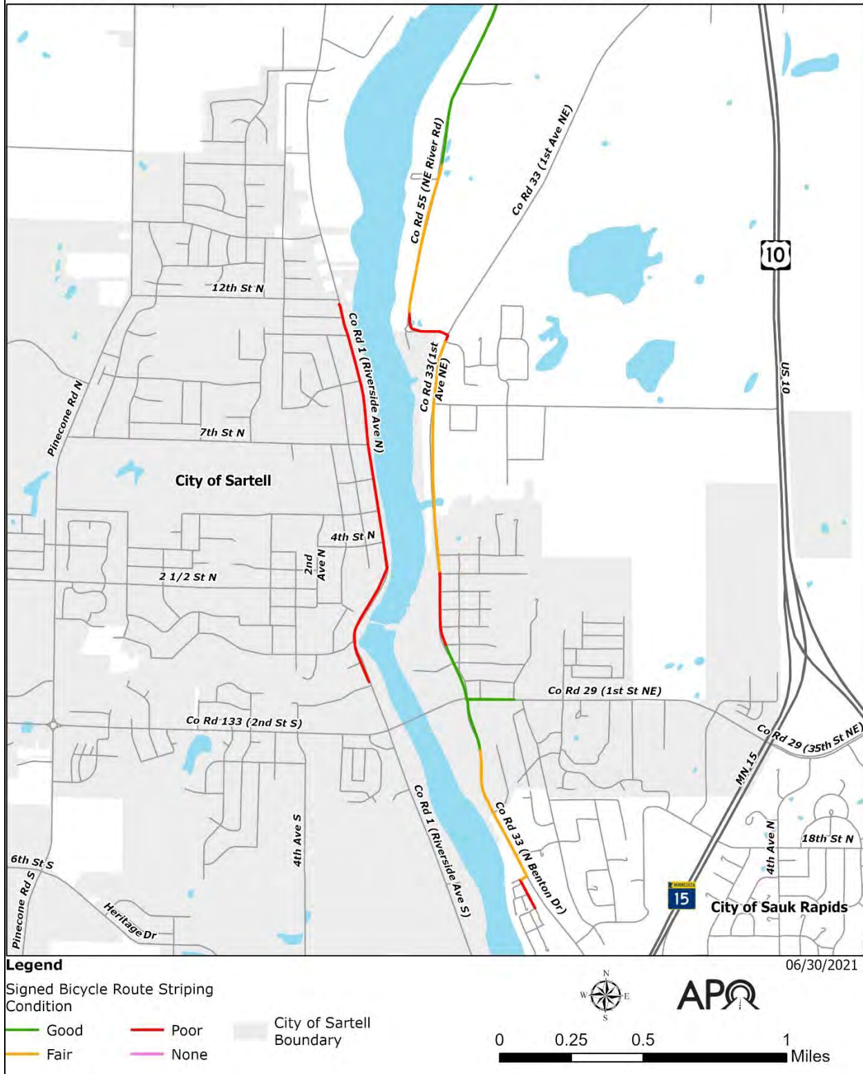
FIGURES B. 10 – STRIPING CONDITION OF ON-ROAD BICYCLE FACILITIES IN NORTH SARTELL.
