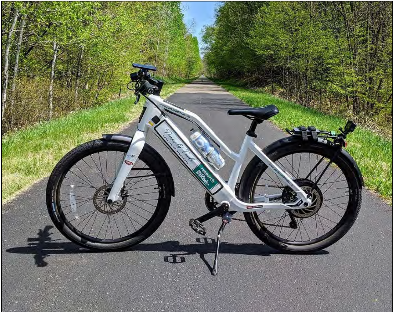
FIGURE 2.22 – PHOTO OF BICYCLE USED BY THE PARKS & TRAILS COUNCIL OF MINNESOTA TO COLLECT PAVEMENT CONDITION DATA FOR SHARED USE PATHS WITHIN THE MPA. PHOTO COURTESY OF THE PARKS & TRAILS COUNCIL OF MINNESOTA.
