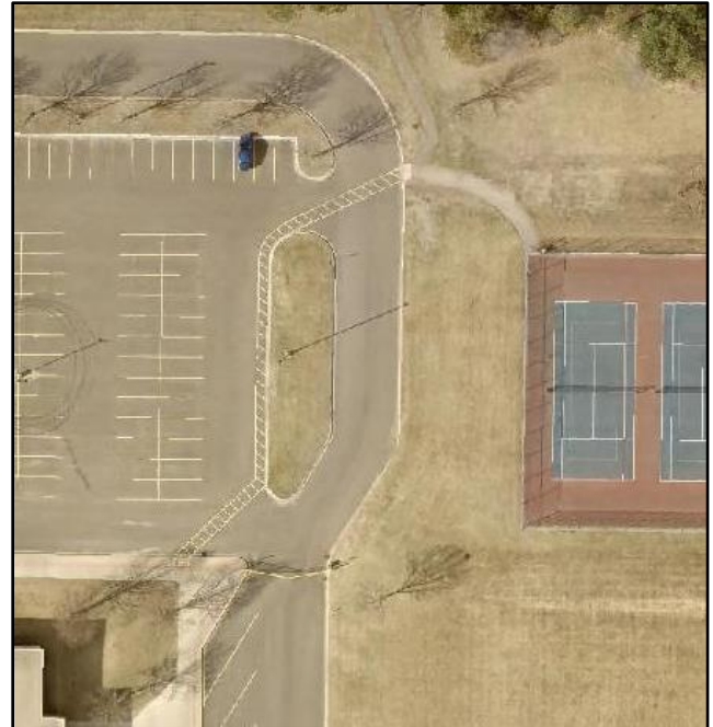
Figure 33. Example of hatched pavement markings through staff parking lot.
