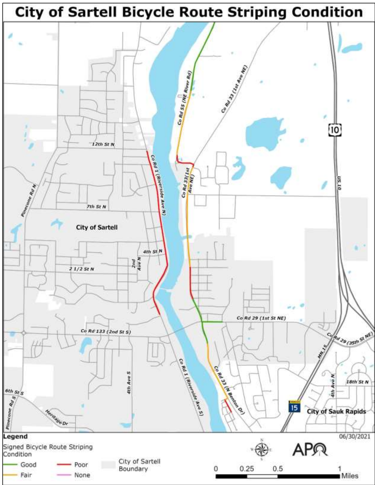
FIGURES B.10 – STRIPING CONDITION OF ON-ROAD BICYCLE FACILITIES IN NORTH SARTELL.
