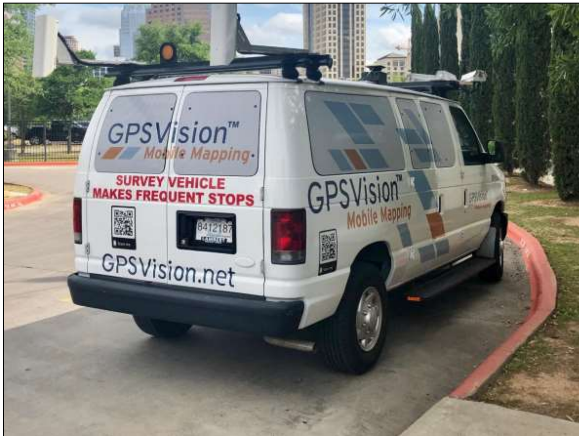
FIGURE 2.21 – EXAMPLE OF DIGITAL INSPECTION VEHICLE.
