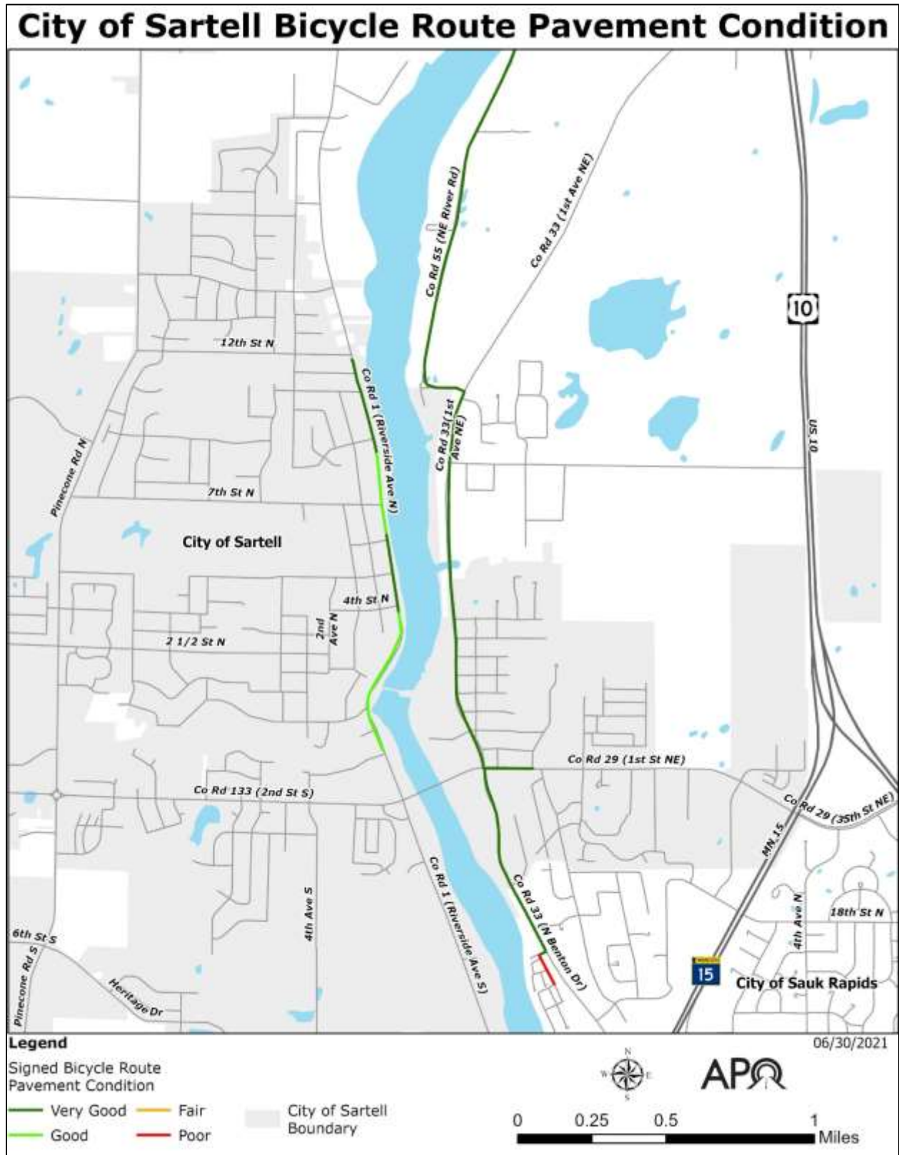
FIGURE B.9 – CONDITION OF PAVEMENTS SIGNED AS BICYCLE ROUTES IN NORTH SARTELL.
