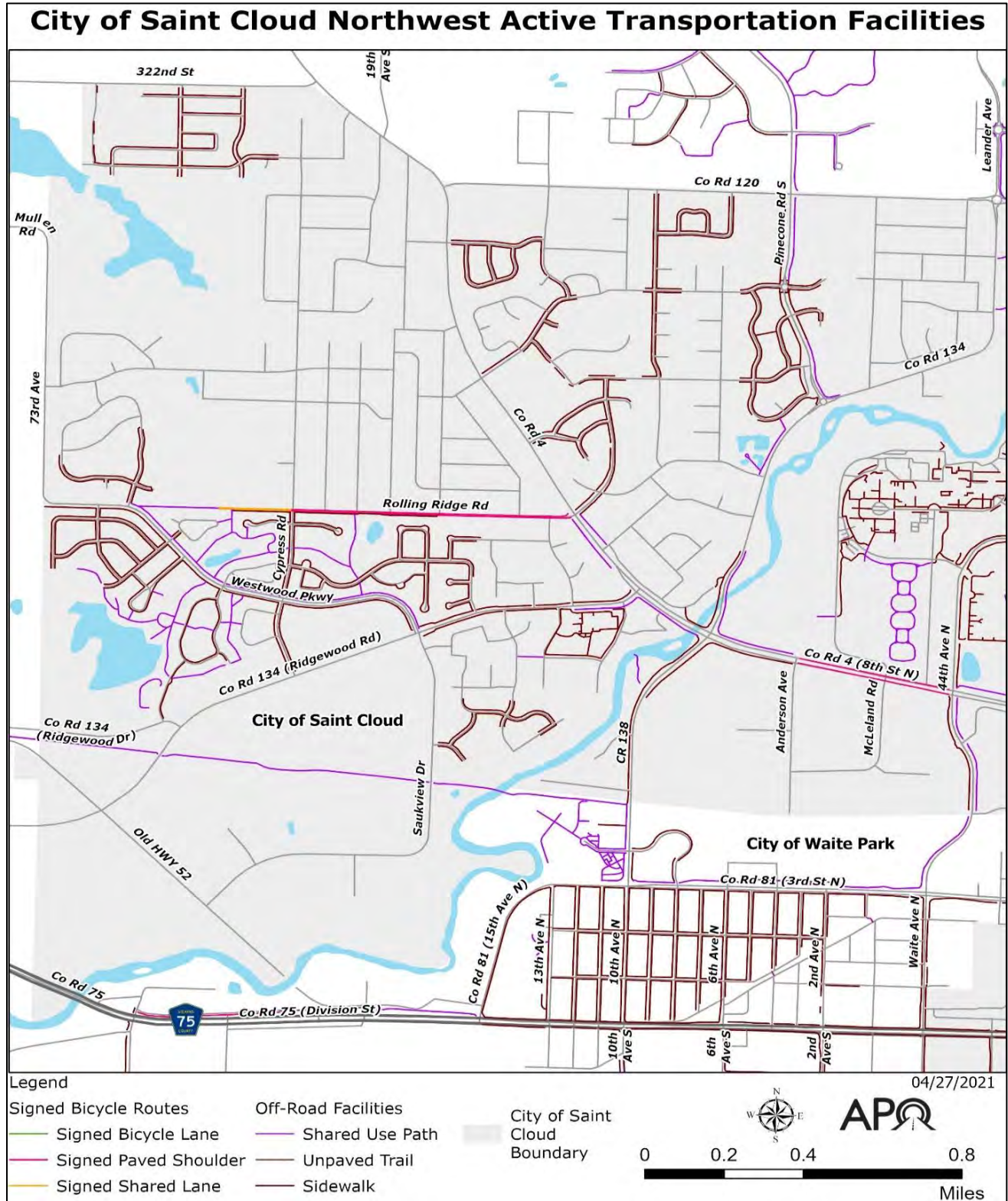
FIGURE E.10 – ON- AND OFF-ROAD ACTIVE TRANSPORTATION FACILITIES IN THE NORTHWEST AREA OF SAINT CLOUD BY TYPE AND LOCATION.
