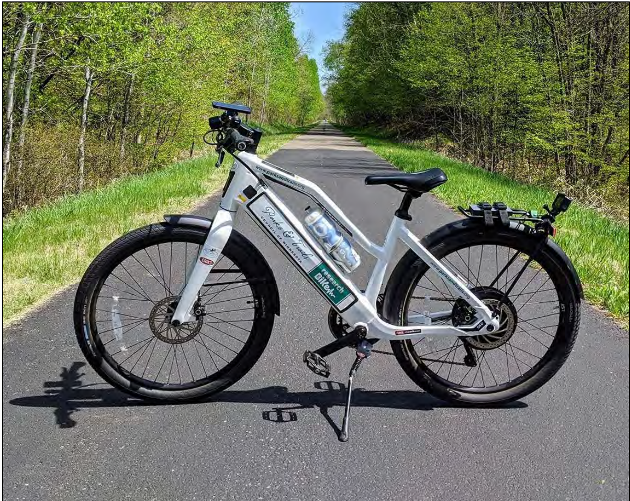
FIGURE 2.22 – PHOTO OF BICYCLE USED BY THE PARKS & TRAILS COUNCIL OF MINNESOTA TO COLLECT PAVEMENT CONDITION DATA FOR SHARED USE PATHS WITHIN THE MPA.
