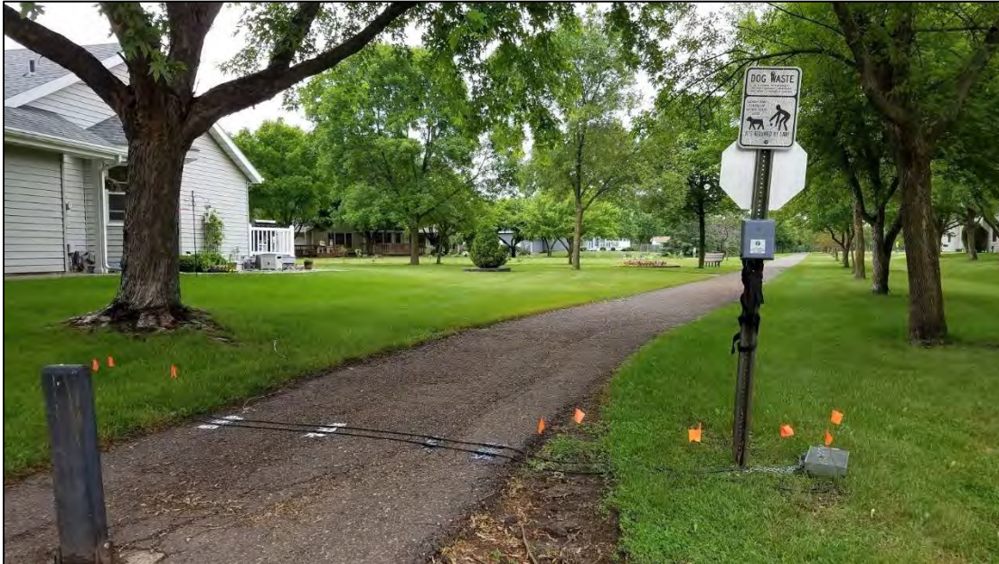
FIGURE 3.26: A PHOTO OF THE TUBE COUNTER AND THE PYRO-BOX COUNTER DEPLOYED AT THE GREENWAY TRAIL IN SAINT CLOUD.
