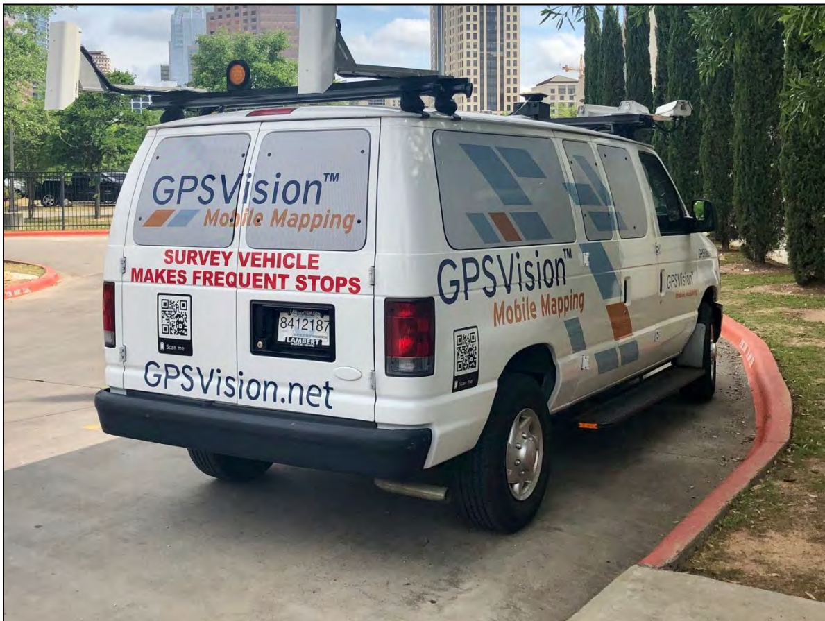
FIGURE 2.21 – EXAMPLE OF DIGITAL INSPECTION VEHICLE.
