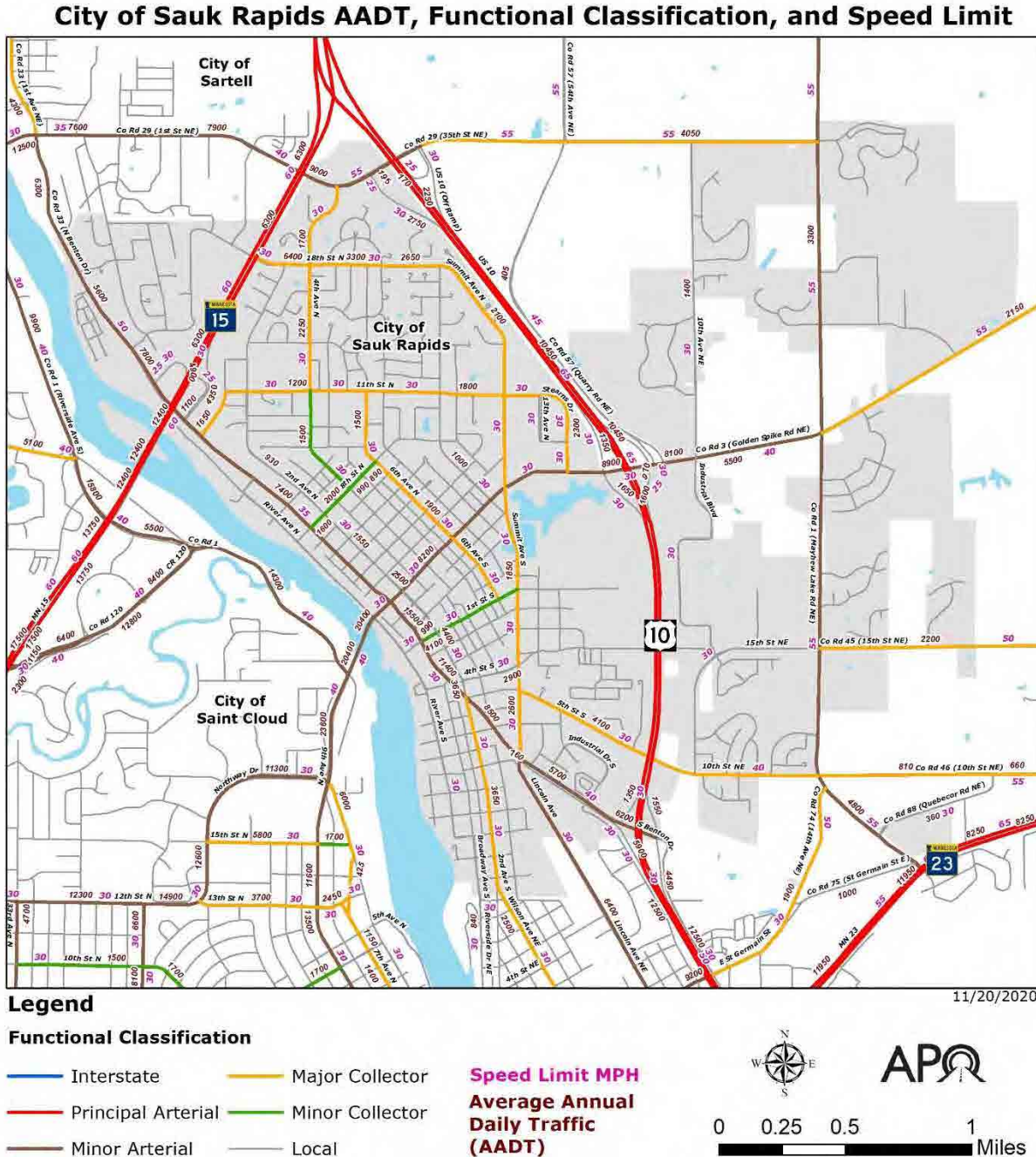
FIGURE 4.7 EXAMPLE OF ROADWAY FACILITY AND USAGE DATA CONSULTED IN FOCUS AREA ANALYSIS
