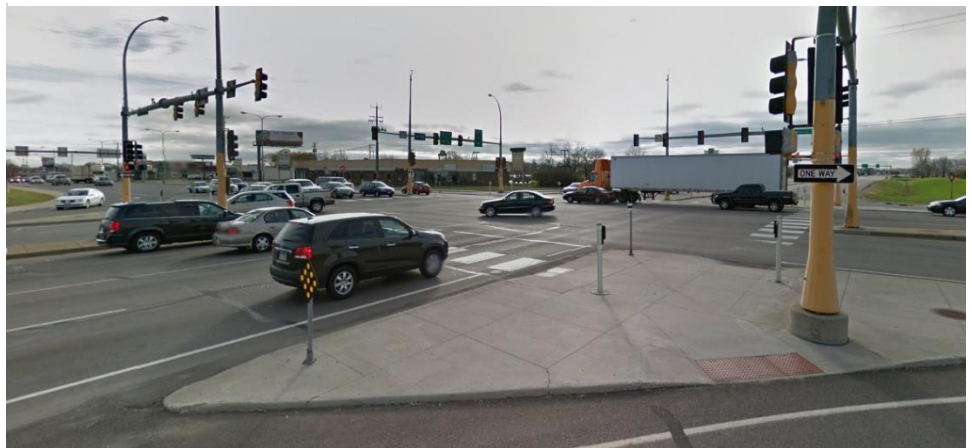
Figure 17 - Minor Approach Channelized Right-Turn at TH 15 and Division Street
